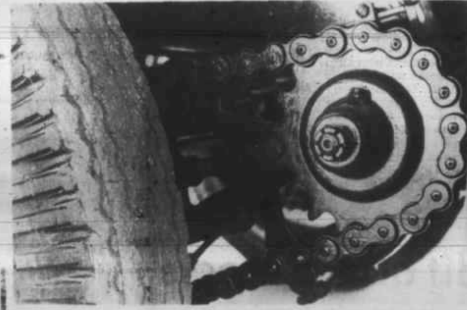
A large chain drive transferred power from the engine to the rear wheels to drive the truck.
