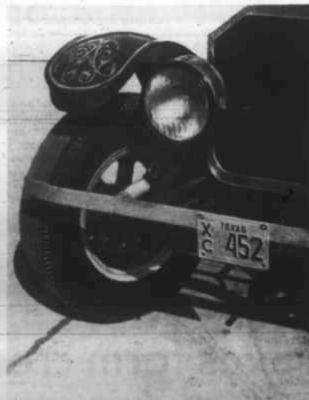
The front bumper of the 1924 truck was spring mounted to absorb shocks. Such a feature on today's automobiles is "new." The hand crank in the lower right of the photo still works.
